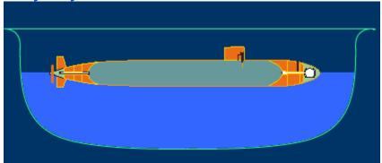
Here we have a toy submarine floating in a bathtub. It's a really fancy sub, made out of steel. The sub weighs one pound. When completely submerged, it displaces two pounds of water.
