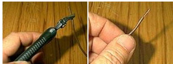
cut too shallow and have to turn and cut again rather than cut the core and have to start again. Now you should be able to slide the insulation off with your cutters, or pull it off with your fingers. This may sound a tedious method, but in no time at all you will be able to do it in two cuts and a flick of the cutters.
