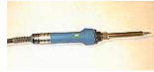
If you have a temperature controlled iron you should start at about 315-345°C (600-650°F). You may want to increase this however - I prefer about 700-750°F. Use a temperature that will allow you to complete a joint in 1 to 3 seconds.
