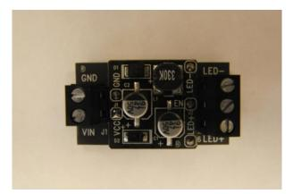
8. Mount the driver in the control box. I used a small piece of butyl rubber tape and just stuck it on the underside of the driver, and then stuck the driver onto the wall of the control box. Done!
