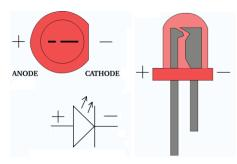
LEDs not only require electricity in the proper direction, but they have somewhat stringent voltage requirements. Diodes don't obey Ohm's Law in a strict sense: current is approximately an exponential function of voltage, so a small change in voltage results in a large change in current. This can be illustrated by a current vs. voltage diagram for an LED.
