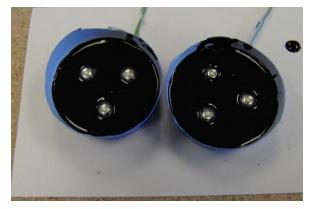
5. Remove the array assembly from the cup. I drilled a mounting hole through the center of the array and attached my headlights to the frame of the ROV using #8 self-tapping metal screws.
