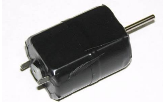
Figure 2.3-1: A Motor Sealed with Electrical Tape
