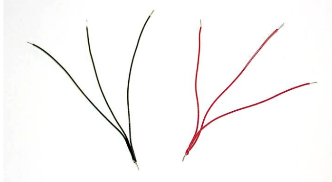
Figure 3.3-3: Spliced Power Wire Bundles
