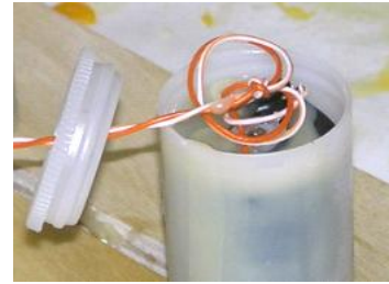
Figure 2.6-12: Wires Coiled in the Top of the Housing, Prior to the Final Wax Pour
