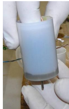
Figure 2.6-8: Settling Motor into Melted Wax at Bottom of Housing
