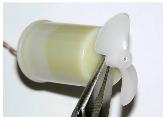
Figure 2.7-4: Propeller and Bushing Mounted on a Motor Shaft
