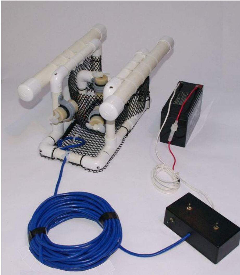
Figure 3.6-3: Completed SeaPerch ROV System, Ready for Testing and Ballasting
