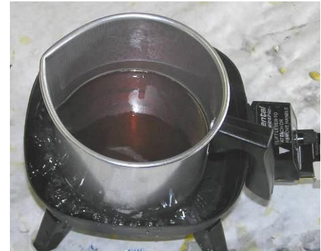
Figure 2.6-3: Wax Melted in Cup in an Electric Skillet with Water to Help Regulate the Temperature
