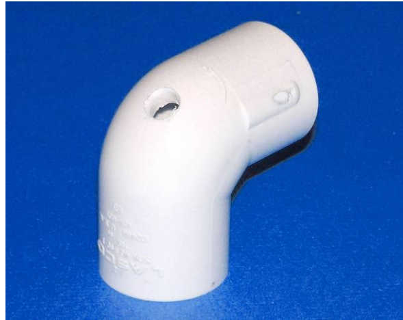
Figure 1.2-1: Drain Hole Drilled in a PVC Elbow
