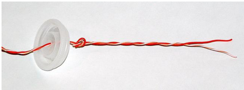
Figure 2.5-3: A Motor’s Wires Passed Through a Thruster Housing Cap
