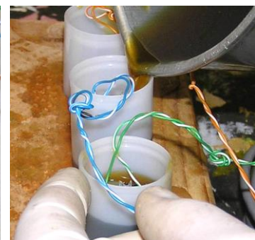
Figure 2.6-11: Wax Filled to ½" from the Top of the Thruster Housing
