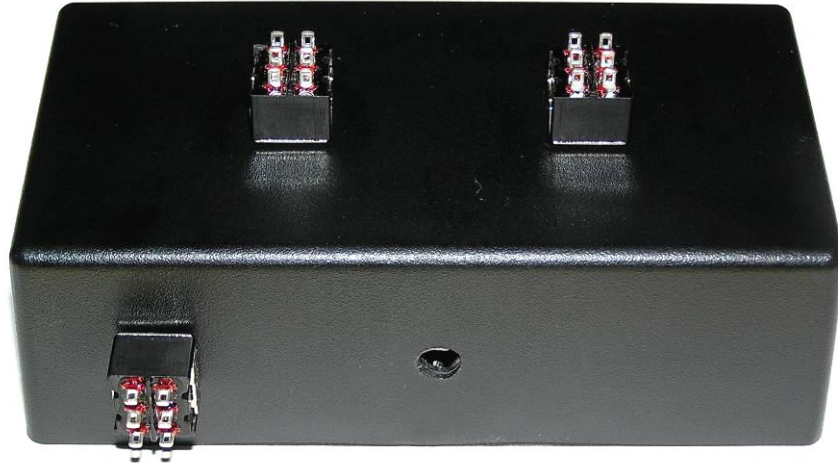
Figure 3.3-8: Control Box Used as a Temporary Switch Wiring Fixture
