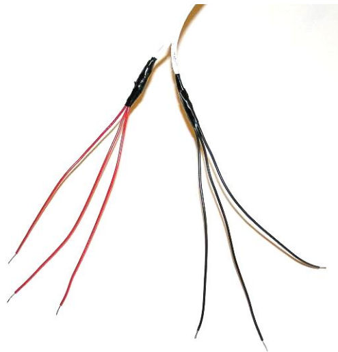
Figure 3.3-7: Wire Bundles Soldered to Control Box End of the Power Cord
