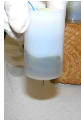
Figure 2.6-9: Wax Moved Part Way Up Around Motor
