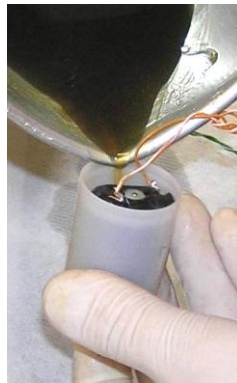
Figure 2.6-7: Pouring Initial ¼" of Melted Wax into Housing
