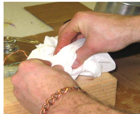
Figure 2.6-15: Using a Paper Towel While Capping the Thruster Housing May Prevent Wax from Squirting Onto You or Others
