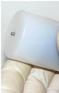
Figure 2.6-5: Motor Shaft Tip Inserted into Hole in Housing
