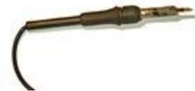
I do not recommend soldering guns, as these have no temperature control and can get too hot. This can result in damage to circuit boards, melt cable insulation, and even damage connectors.
