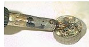
Some solder stations come with a little pad at the base of the holder. If you have one of these, you should get into the habit of wiping the tip on the pad each time you apply solder with it.
