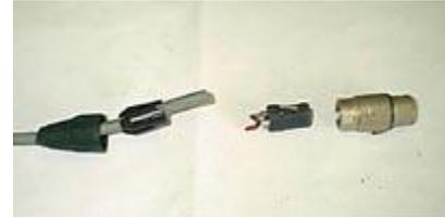
Once you have all the connector parts on that you need, you will need to strip your cable. This means removing the insulation from the end of the wire and exposing the copper core. You can either use a wire stripper, side cutters, or a knife to do this.
