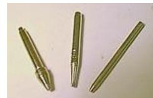
'spade tips'). If you have a solder station with a desolderer, you will also want a range of desoldering tips and cleaners.
