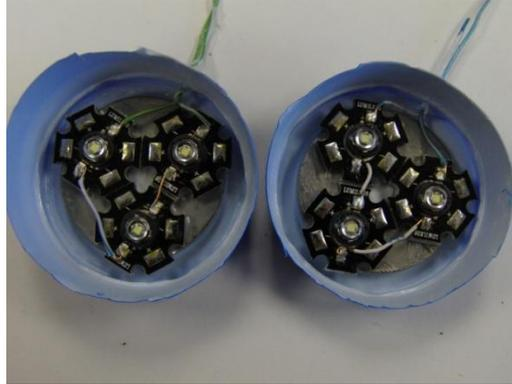
4. Mix up a batch of your epoxy according to manufacturer's directions and carefully! pour the epoxy into the bottom of the cup so it just covers the electrical contacts on the face of the LEDs. Be sure the junction where the LED lens meets the body is covered, but do not cover the lens. Let it cure for the specified time.
