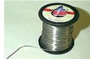
Rosin core solder comes in three main types - 50/50, 60/40 and 63/37. These numbers represent the amount of tin and lead present in the solder, as shown below.
