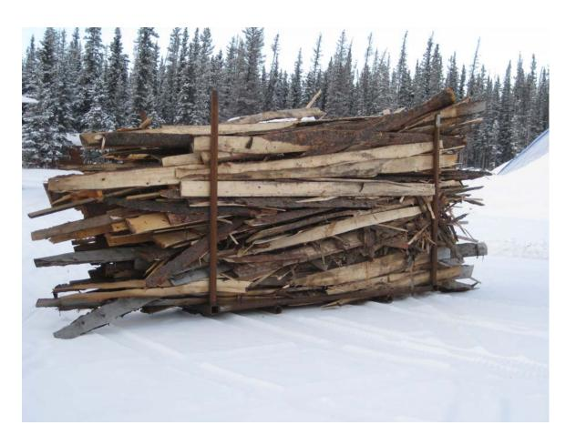
Hemlock jacket boards, slabs and edgings were saved for this research project and were dried in make-shift racks in a lumber dry kiln to approx -imately 5% MC (db).
