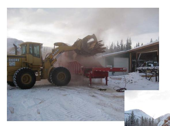
Kiln-dried slabwood of each species was reduced to "hog fuel" in with a Rotochopper MC266 horizontal grinder.
